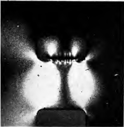
Fig. 12. Photographs of strain pattern produced by 650-g load on perforation edge.
